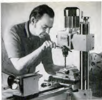
FOR DRILL-PRESS WORK , compound slide is unbolted from carriage worktable, replaced by machine vise
